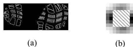
Figure4. Result of the co-occurrence matrix. (a) The edge points of an input shoeprint image. (b) An gray-level representation of  $CM$
