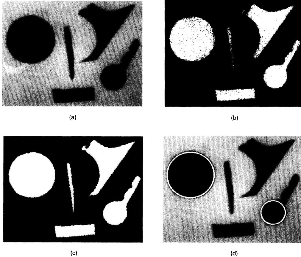
**Fig. 7** Result of applying the proposed method to a noisy real image: (a) a noisy image, (b) the result of applying the entropy-based thresholding method to (a), (c) the result of applying the noise-cleaning filter to (b), and (d) the final result of the proposed method.
