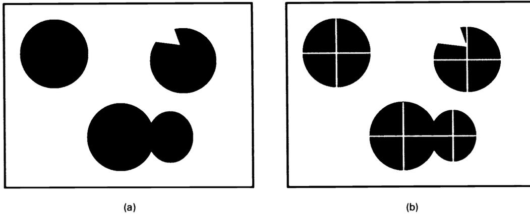
**Fig. 5** Result of applying the proposed method to a synthetic image: (a) a synthetic image and (b) the result of applying the proposed method to (a) with each white line segment standing for a diameter of the detected circular objects.
