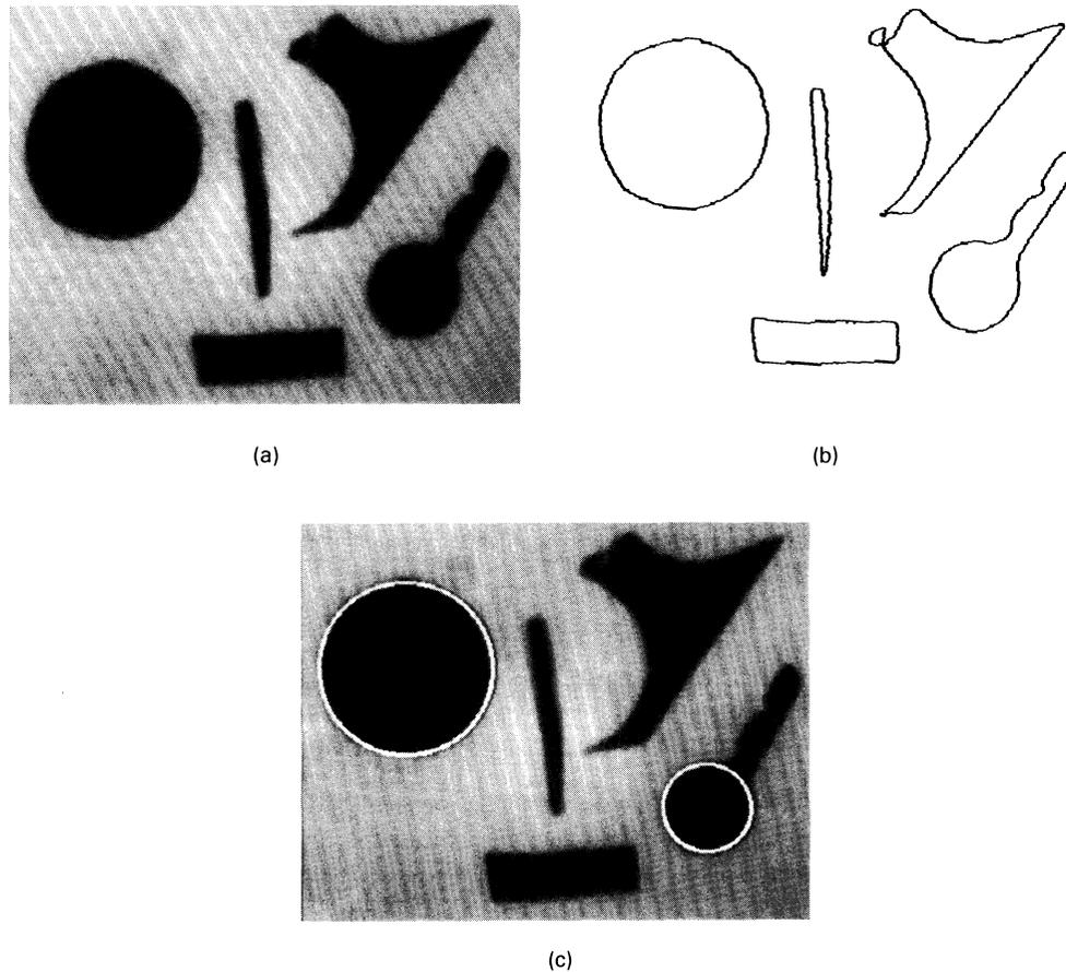
**Fig. 6** Result of applying the proposed method to a real image: (a) a real image, (b) the result of the boundary extraction, and (c) the final result of the proposed method with two white circles standing for two extracted circular objects (coin and key head).
